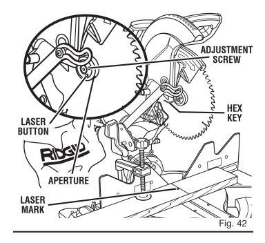
NOTE: When properly aligned, the laser should be on the left edge of the kerf.
